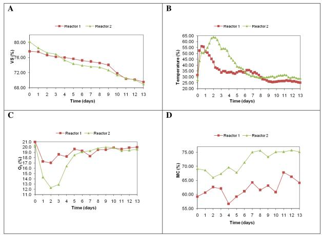
Figure 1. Changes of process parameters during the process: a) volatile solid content, b) temperature, c) oxygen concentration, d) moisture content.
