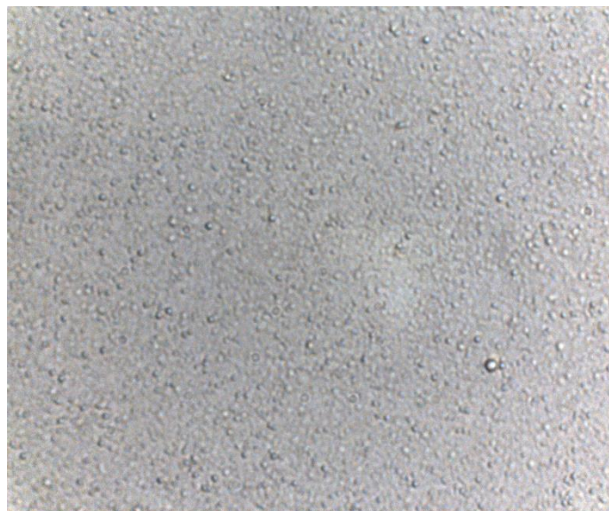
Figure 1. Liposomes under microscope at a magnification of 100 x (small round creatures are actually formed liposomes of different sizes)
